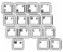
To activate the keypad, press the Num Lock key. The 15 keys shown in the figure switch from alphabetic keys to numeric keys. Press Num Lock again to return to alphabetic.
